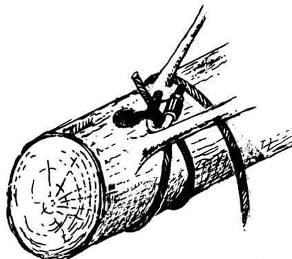
Figure 2 . Wrapping and Clamping Cable to Tree Trunks
