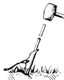
Figure 4. Driving a Duckbill Earth Anchor
