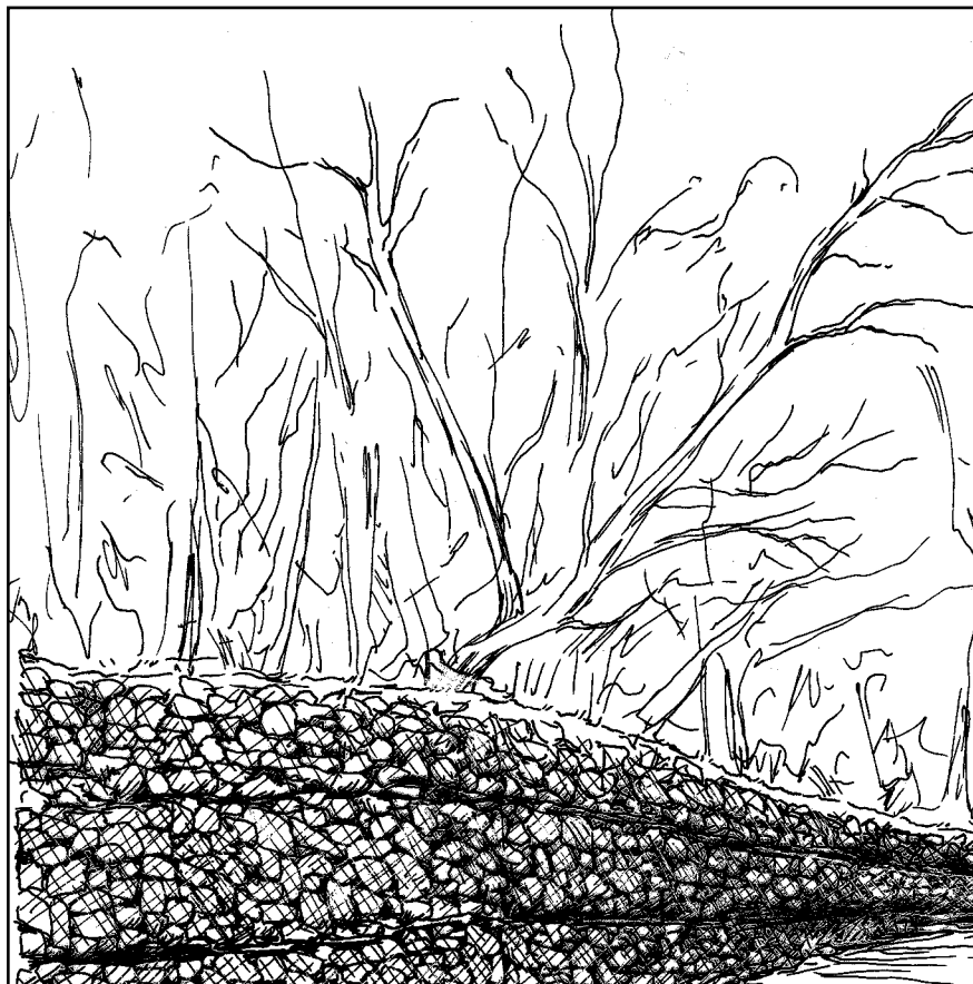
Figure 1. Gabion revetment on streambank
