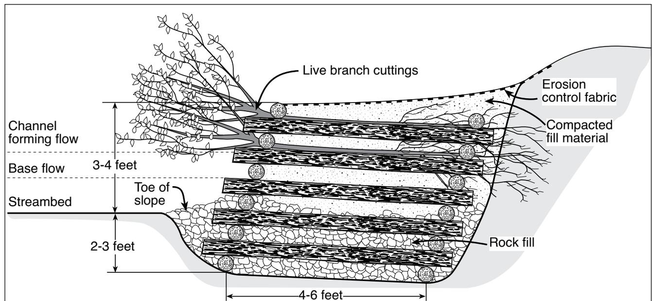
Figure 1. Cross section of a live cribwall.
