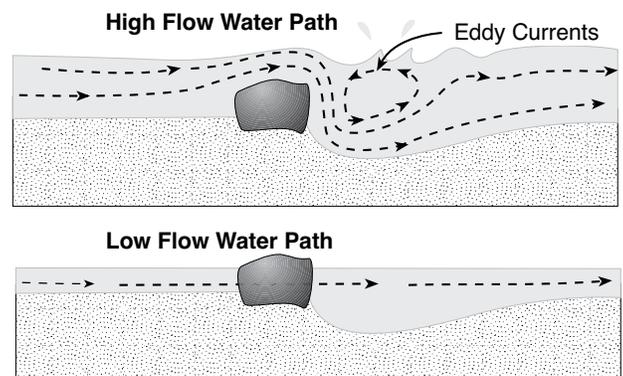
Figure 2. Effects of Flow Levels on Eddy Currents
